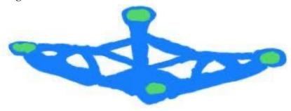
The example shown above is a sketch of a proposed topology optimized drone that can be fabricated using FDM additive manufacturing. The preliminary sketch shows what the drone may look like if it were topology optimized. Note the body shows a truss-like structure which is a signature of topology optimization and it is not a shape that can be manufactured efficiently through traditional manufacturing methods which makes it a prime candidate for the application of additive manufacturing.
