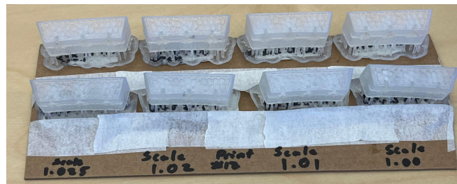
Figure 10: Shift Keycaps at varying scales (top row is cured, bottom row is uncured).
